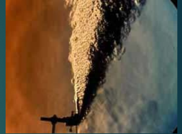
Schlieren image of Helium flow (courtesy of Floviz)
